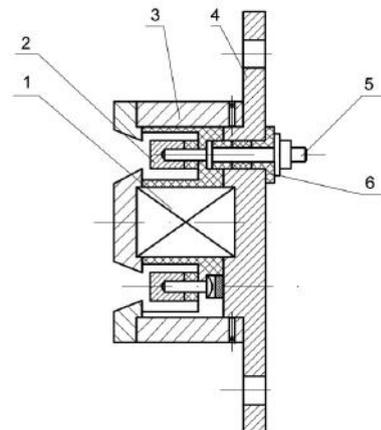
**Fig. 1.** The ion source with a cold cathode and a divergent flow of plasma gas discharge
