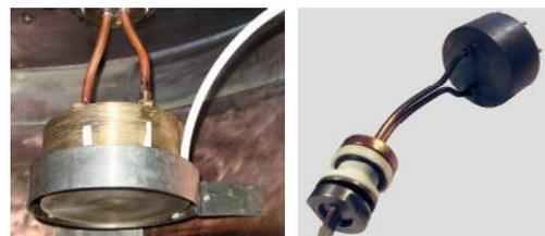
**Fig. 5.** Photos of magnetron sputtering devices
